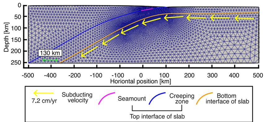
**Figure 3.** Numerical domain and mesh.
